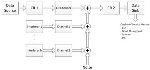
Figure 2. Example configuration for CR test infrastructure (reverse channel from CR2 to CR1 omitted for clarity)
